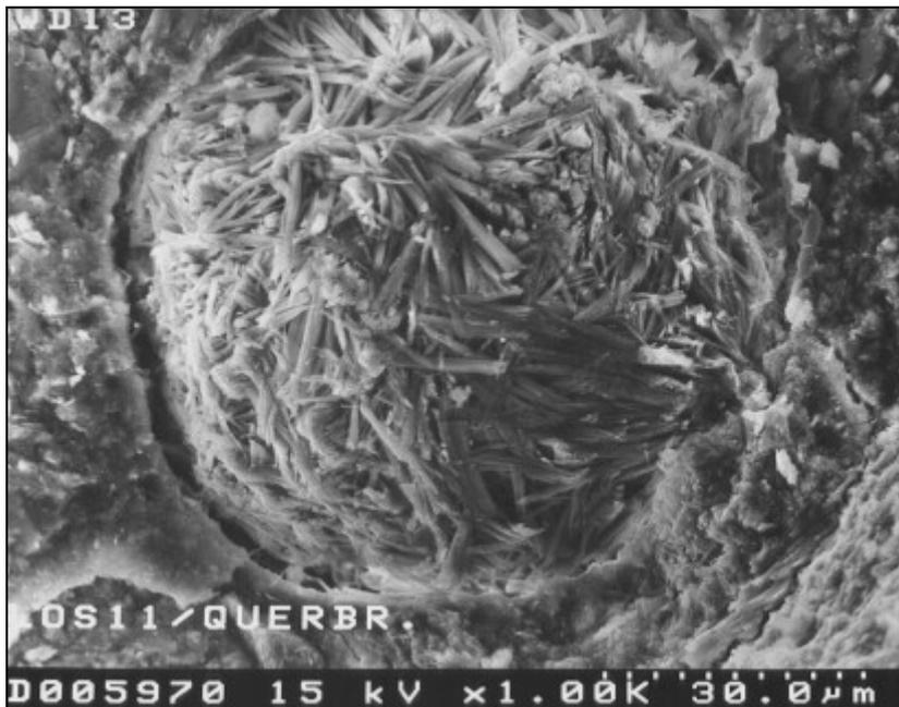
Fig. 16: Air void completely filled with ettringite crystals in a damaged pavement concrete
