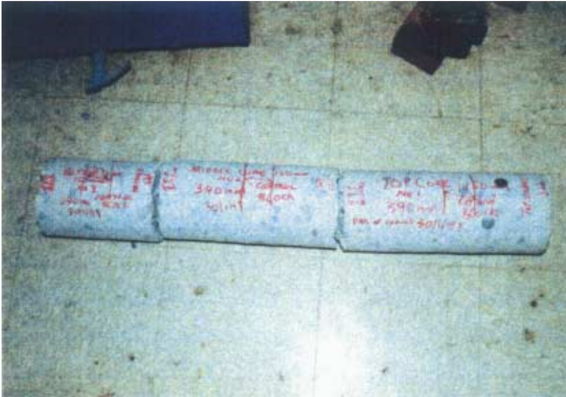
Photograph 3: Shows one set of \text{\O} 150 \times 900\text{mm} core after coring.
