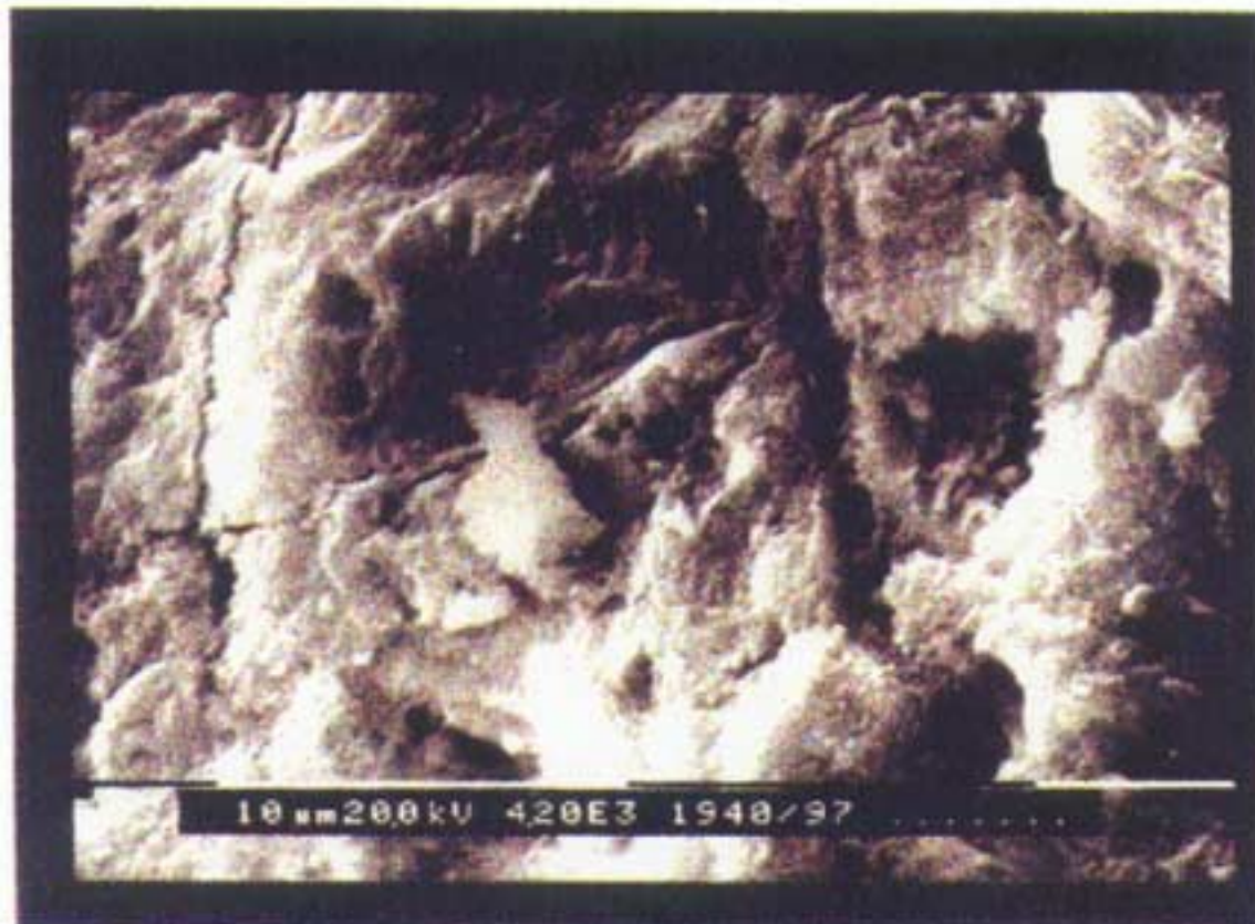
Photographs 5 & 6: SEM on control concrete at 28 days.
