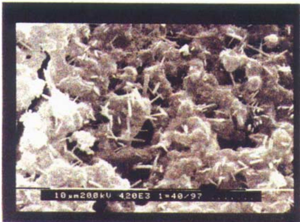
Photograph 7 & 8: SEM on treated concrete with XYPEX Admix C-2000 Waterproofing at 28 days.
