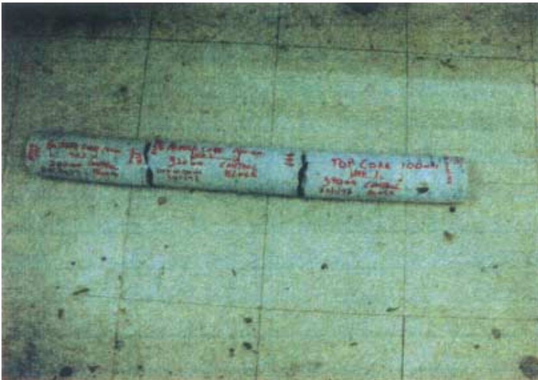
Photograph 2: Shows one set of \text{Ø } 100 \times 900\text{mm} core after coring.
